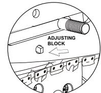
7. Ensure that the adjusting block is located in the tensioning hole on the chain bar.
