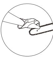
11. Tighten until there is enough play that the chain can be pulled away from the bar, but not so much that the runners can be pulled out of the bar.
