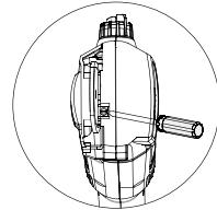
1. Release chain tension by turning the tensioning screw, located behind the chain bar, counter-clockwise.
