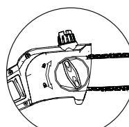
12. Once you have the correct tension, fully tighten the locking knob.
