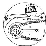
6. To replace the bar and chain, loop the chain over the drive pulley and place the bar against the centre alignment groove.
