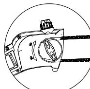
9. Replace the side cover and locking knob, but do not tighten.
