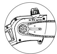
4. The bar and chain can now be removed by lifting it away from the main body of the saw and releasing the chain from the drive pulley.
