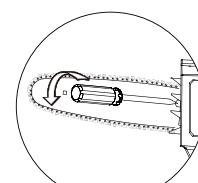
10. Using a screwdriver on the tensioning screw, turn clockwise.
